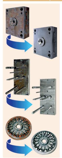
The VST Line for ultrasonic mold cleaning covers every cleaning and protection need, in order to eliminate contaminants and preserve the mold from possible oxidation until its next use.
