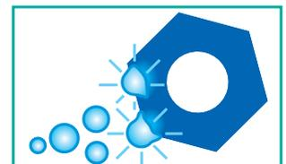
④ During the pressure phases, the bubbles implode when they come into contact with the immersed parts and release the energy that created them. This mechanical energy also improves the efficiency of the chemical action of the cleaning product used in the tank.
