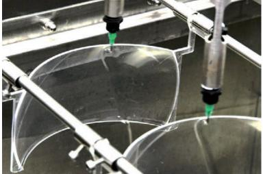
Permanent verification of the outflow and the pressure on the nozzles, ideally completed with the **FISA Autocoat** device ensure regular and even application of coating.
