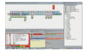
As for the **FISA LOGGER**, it collects and saves all the process data depending on the baskets of parts currently in the machine to enable you to keep a record for each production batch (temperature, time, ultrasonics etc). It is also equipped with a maintenance management system capable of indicating maintenance operation dates: replacement of detergent products, filtering media or cartridges etc
